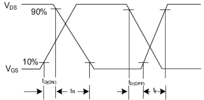
Fig. 2.2 Switching Waveforms
